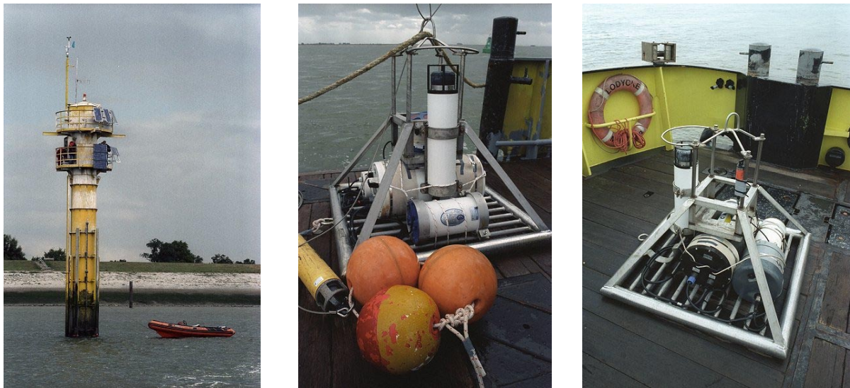
Fig.1: Example system with master unit (on measurement pole) and two slaves units (before deployment)
